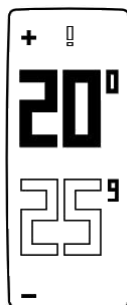
Exclamation mark: Relay not detected (loss of radio synchronization between Thermostat and Relay)
