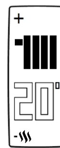
Radiator logo: a Valve located in a different room than the Thermostat requires heating
